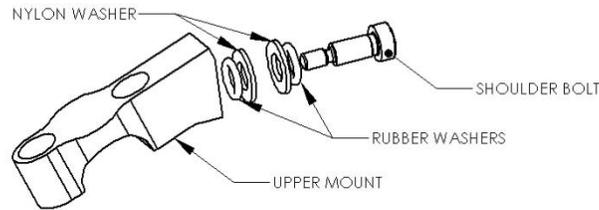
17. Test the assembly by tightening the 8mm screw. If excessive force is required to accomplish this, or if any of the mounting surfaces contact or bind, remove floating mount and refer to step 14. This should also be inspected after riding to insure proper operation.
